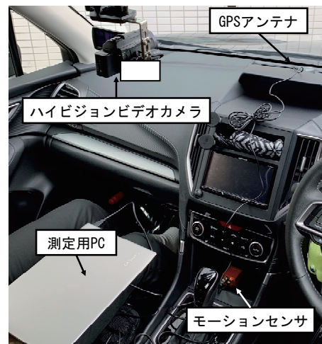
Fig 5 Installation of equipment and materials
