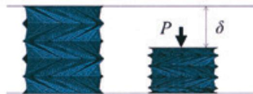
(c) Deformation simulation by FEM analysis
