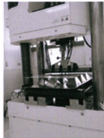
Fig.11 Hydraulic system universal testing machine
