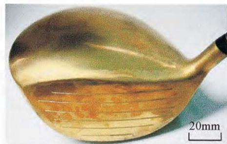
Fig.14 Outline of golf head after endurance test.
